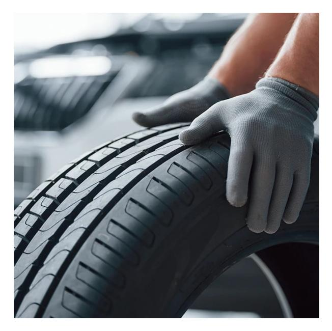
Winter driving requires adequate traction for safe manoeuvring on slippery surfaces. Check your tire tread depth and condition. If the tread is worn, consider replacing your tires or switching to winter tires for improved grip. Winter tires are designed with special rubber compounds and tread patterns to enhance traction in cold conditions. Don't forget to maintain the recommended tire pressure for optimal handling and fuel efficiency.
