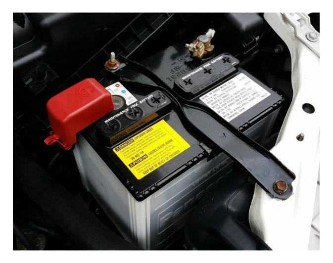
Cold weather can significantly impact your battery's performance. Clean the terminals and ensure they are tightly connected. Have your battery tested to ensure it holds a strong charge. If necessary, consider replacing it with a <u>high-quality battery</u> from Leicester Motor Spares to avoid unexpected breakdowns.
