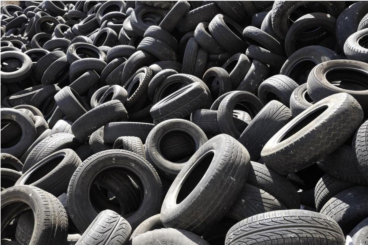
Used tyres may be replaced with remoulded or retreaded tyres. Retreading is replacing the rubber on the carcass of a previously used tyre. As long as the tyre is in good condition and free of punctures and other damage, this method serves its intended purpose well. [Budget tyres](#) are another possibility.
