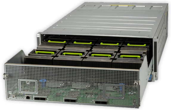
Figure 3. The Supermicro X12 Gaudi AI Training System, powered by Habana Gaudi processors and 3rd Generation Intel Xeon Scalable processors, features 64 Habana TPCs and up to 8 TB of DDR4-3200MHz memory
